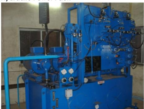
All LF movements are powered hydraulically. For smaller capacity LF, Low pressure water hydraulic system is employed while for larger capacity, just one single compact power pack unit is used, operating at a pressure of about 100 bar.
